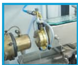
1ST EXTRUDER equipped with gravimetric control system (inner layer formation)
