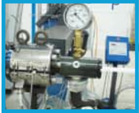
2ND EXTRUDER (glue) equipped with gravimetric control system
