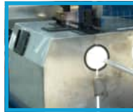
ALUMINIUM WELDING UNIT check of parameters and visual verification of the same with telecameras
